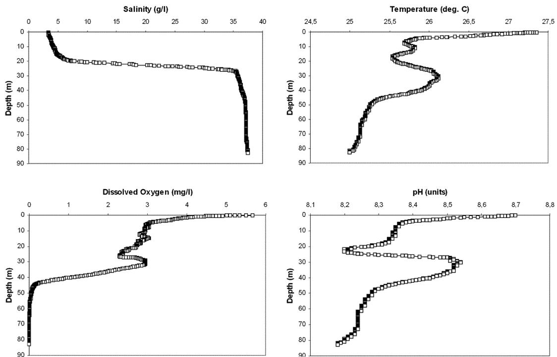
**FIGURE 8.** Salinity, temperature, dissolved oxygen, and pH water column profiles from Stargate Blue Hole, South Andros, Bahamas, taken on 20 August 1997 with an YSI Model 600XLM multi-parameter water quality monitor. Squares represent individual data points.
