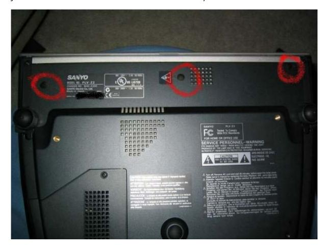
Step 2: Then remove the three screws on the back panel.
